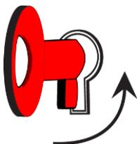
Turning the keyswitch (if enabled) anticlockwise to the horizontal (I) position gives the user instant entry to access level 2.
