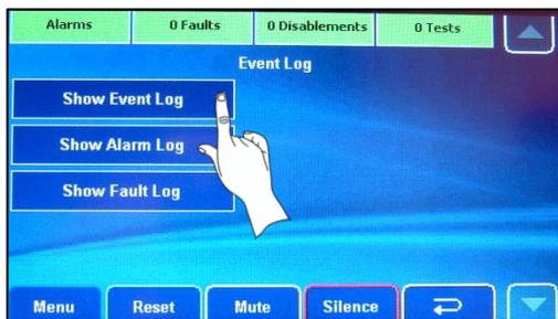
The **Show Event Log** button, when pressed, lists both the panel's event and alarm log (up to 9,999 events). This includes fire, fault and system events.
