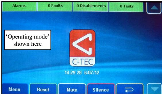
Under normal operating conditions (shown left), with no fires, faults or pre-alarms present, a message may be displayed on the touchscreen indicating the current operating mode of the panel. The operating mode is programmed by an authorised systems engineer and is defined by the client/system specifier. Refer to your system specifier's documentation for further details.
