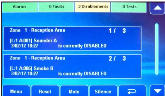
If there are more than one disablement, the top right corner of the display will show, for example “1 / 3” and can be scrolled through using the and buttons, or by using the scroll bar.
