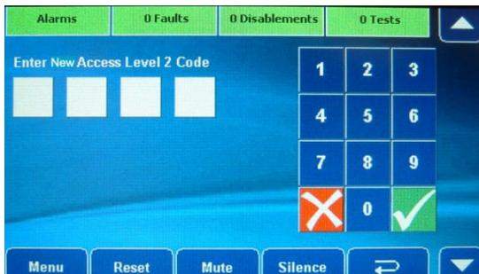
Use the numeric keypad buttons to enter the new access level 2 code. After the fourth digit has been entered, the panel will request you confirm the new code by re-entering it.
