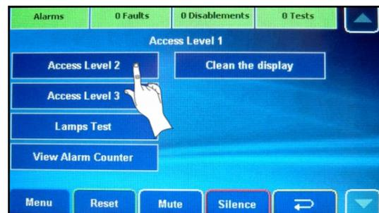
Press the **Access Level 2** button and the display shown below appears:
