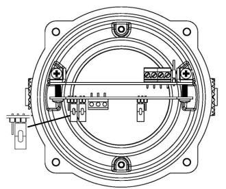
J2 Header Pin - Postion B (pins 2 & 3 linked) places power supply TB Fault resistor & RLY 1-2 in
