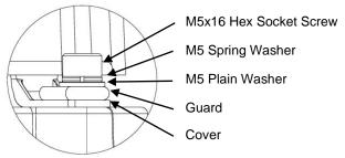
Fig. 13 Cover and Guard Fixtures
