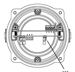
J7 Header Pin - <u>Postion A</u>, Factory default position (pins 2 & 3 linked) set to normal operation.
