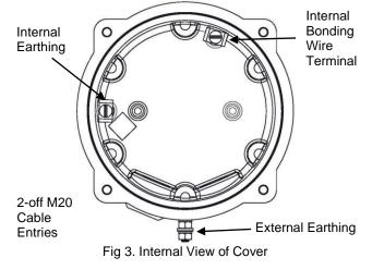
When using the internal earth terminal ensure that the stainless steel M4 flat washer is between the incoming earth wire and the enclosure.
