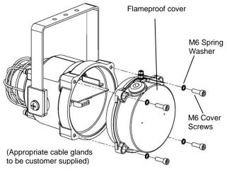
Fig. 2 Accessing the Explosion proof Enclosure.
