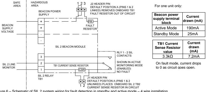
Figure 6 – Schematic of SIL 2 system wiring for fault detection in standby and active mode – 4 wire installation
