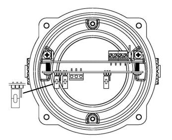
J2 Header Pin - Postion A, Factory default position (pins 1 & 2 linked) removes power supply TB Fault resistor & RLY 1-2 out of circuit.
