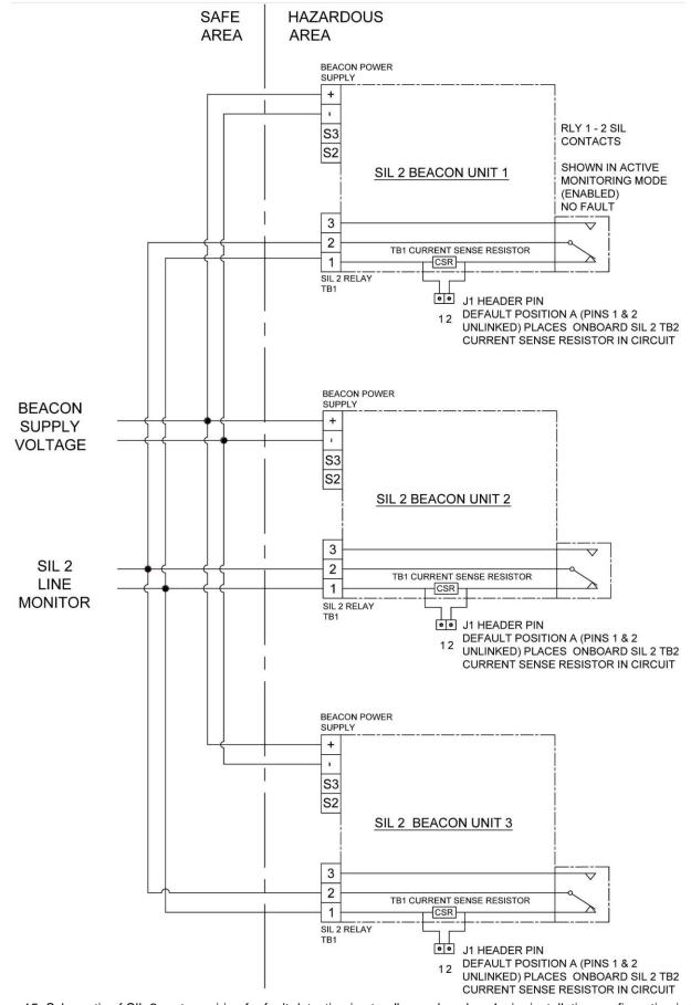
Figure 15: Schematic of SIL 2 system wiring for fault detection in standby mode only – 4 wire installation configuration in Star formation
