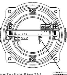
J7 Header Pin - <u>Postion B</u> (pins 2 & 3 linked) set for hard reset.
