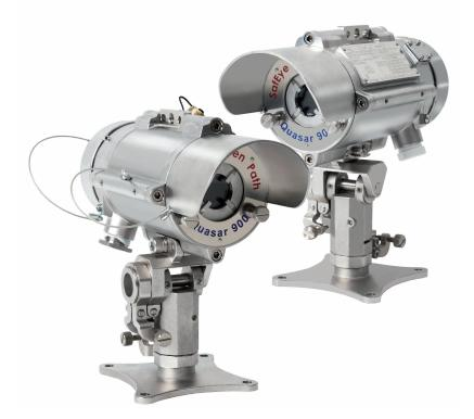
The SafEye Quasar 900 is part of the innovative SafEye Quasar open path gas detector series. The detector provides continuous infrared technology monitoring for combustible hydrocarbon gases at very low concentrations, up to 95 percent obscuration, featuring advanced wide area coverage with long range detection at up to 660 ft. (200 m) and high-speed response in under three seconds. The SafEye Quasar 900 ensures reliable and accurate protection to keep a SafEye on your safety.
