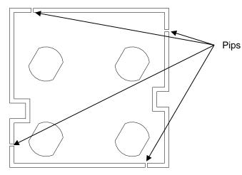
Using a pair of strong side cutters, cut through the 1mm pips of the metal plate as shown below:
