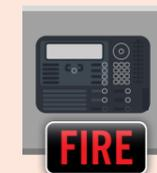
**FIRE** automatically displays on panel. Signal is 'latched' until reset by a **Responsible Person**.
