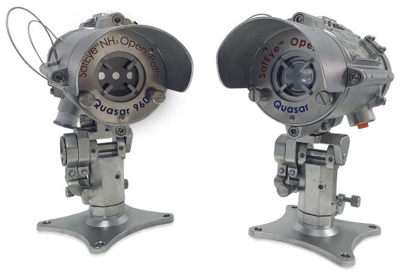
The SafEye Quasar 960 is part of he innovative SafEye Quasar open path gas detector series. The detector provides ultraviolet technology continuous monitoring for toxic ammonia ( $NH_3$ ) gas at very low concentrations, up to 95 percent obscuration, featuring advanced wide area coverage with long range detection up to 200 ft. (60 m) and high speed response in under 10 seconds.
