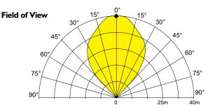
To meet the requirements of EN54:10 clause 5.4, where the ratio of the response points. Dmax: Dmin should not exceed 1.41, the horizontal and vertical viewing angles max should not exceed  $\pm 30^{\circ}$ .
