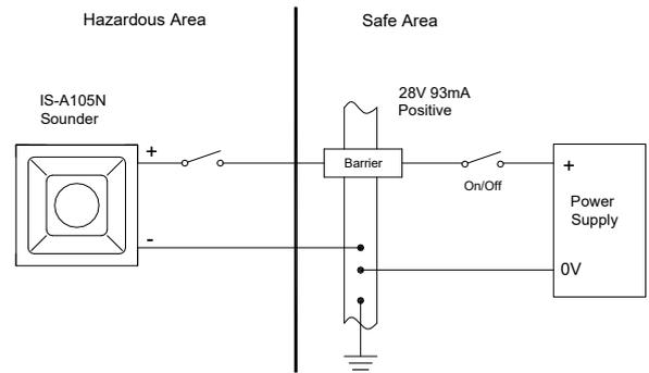
Fig 3 Single stage alarm using single channel barrier.
