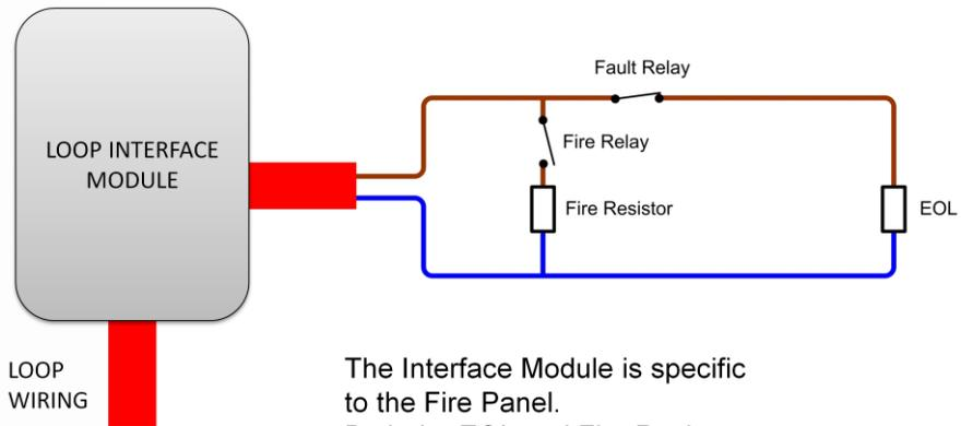
The Interface Module is specific to the Fire Panel.
