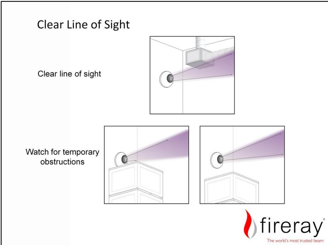
A Beam is an obscuration device and so needs a clear line of sight between the Transmitter and Receiver or Reflector to work effectively. An obstruction during Beam alignment can make a Reflective or Projected Optical Beam difficult to align.
