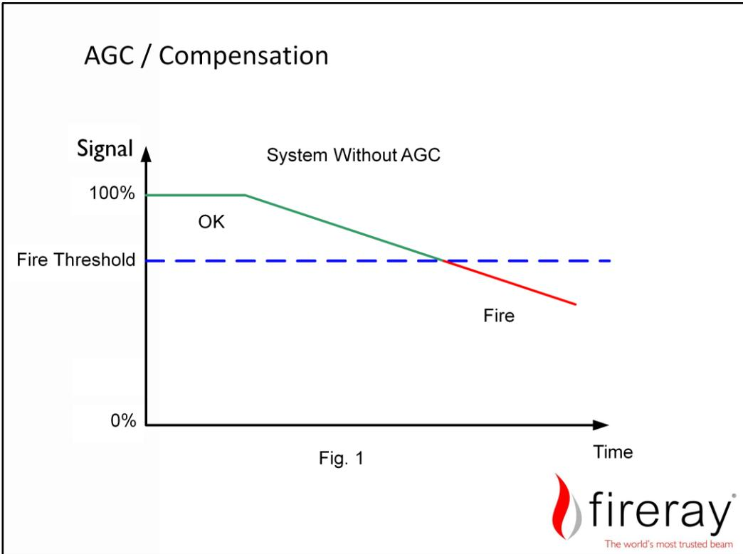
Automatic Gain Control (AGC), as its name suggests, changes system gain to compensate for slow changes in signal level. Such signal level changes may come from gradual dust build up on the Beam lenses and/or from gradual movement of the building, either of which can reduce the signal received by the detector. AGC occurs automatically and does not require user involvement.
