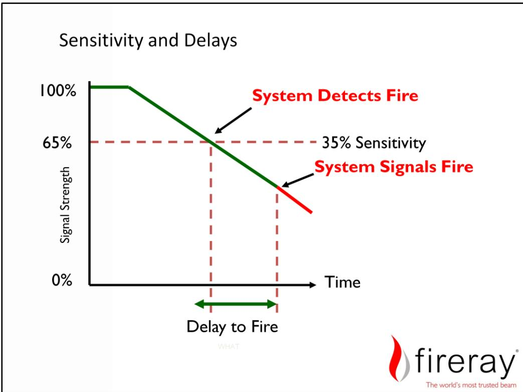
Fireray50R and Fireray100R have sensitivity thresholds of 25%, 35% and 50%, whereas Fireray3000 and Fireray5000 have thresholds selectable anywhere between 10% and 60%.
