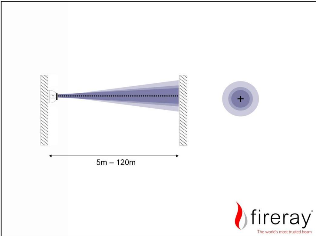
An Optical Beam Smoke Detector is a device that monitors the amount of obscuration present in an open area. It does this by transmitting a beam of infrared light across the area to be protected, and monitoring the amount of light that is received after it has passed through the area. If the light received falls below a predetermined level it is decided that the obscuration (by smoke) has increased to such a level that a Fire must be signalled to the Fire Alarm Control Panel (FACP).
