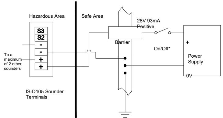
Fig 4 Single stage alarm using single channel barrier.
