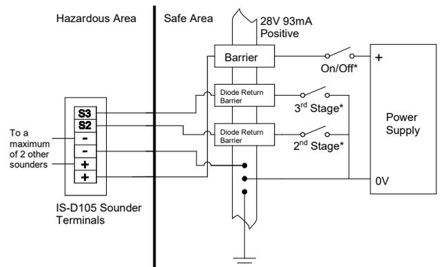
Fig 6 Multi stage alarm using Zener barriers.
