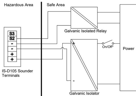
Fig 8 Multi stage alarm using galvanic isolated relays
