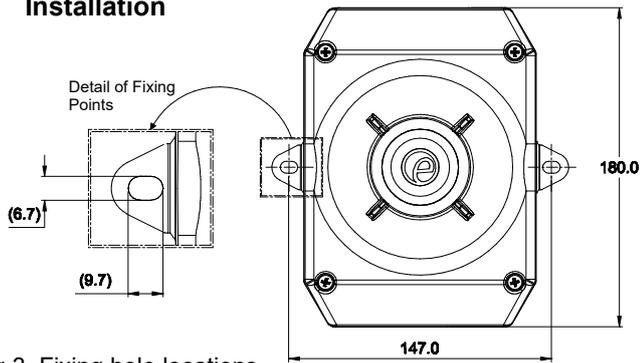
Fig 3 Fixing hole locations
