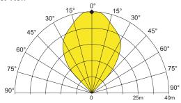
To meet the requirements of EN54:10 clause 5.4, where the ratio of the response points Dmax: Dmin should not exceed 1.41, the horizontal and vertical viewing angles max should not exceed  $\pm 30^{\circ}$ .
