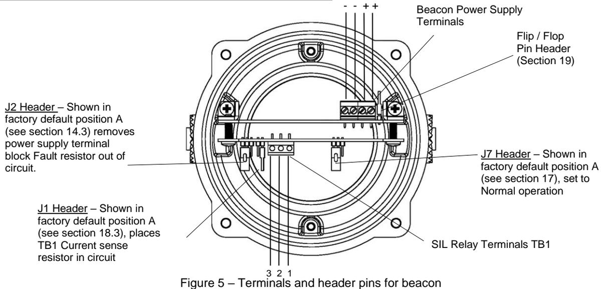
Figure 5 – Terminals and header pins for beacon
