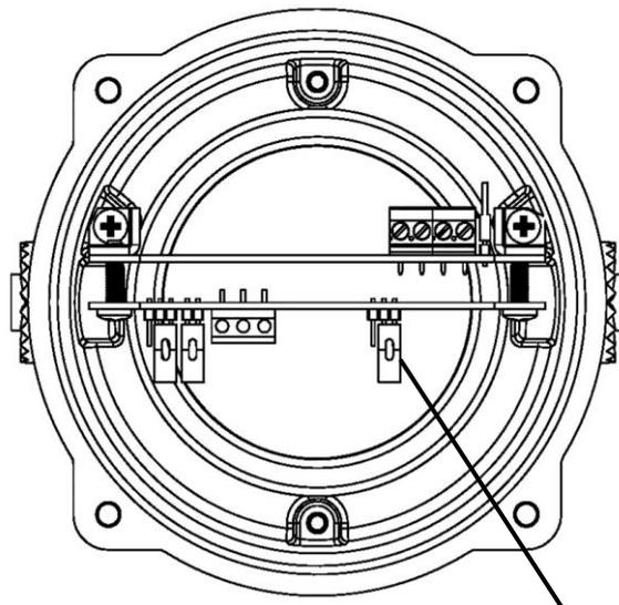
J7 Header Pin - Position B (pins 2 & 3 linked) set for hard reset.
