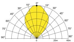
To meet the requirements of EN54:10 clause 5.4, where the ratio of the response points Dmax: Dmin should not exceed 1.41, the horizontal and vertical viewing angles max should not exceed ±30°.
