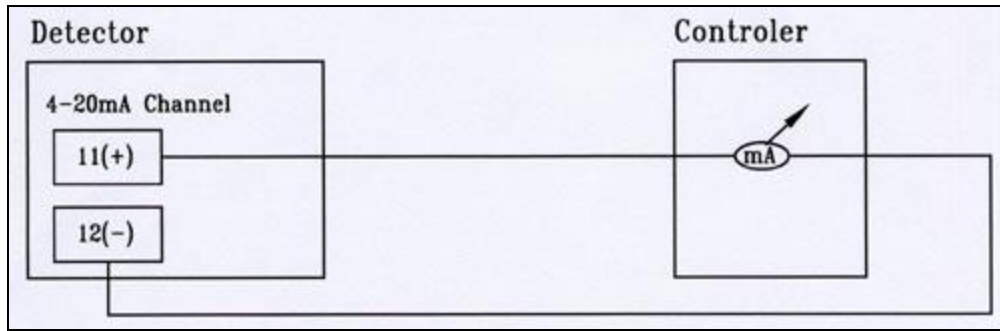
Figure 21: 4-20mA Source Output
