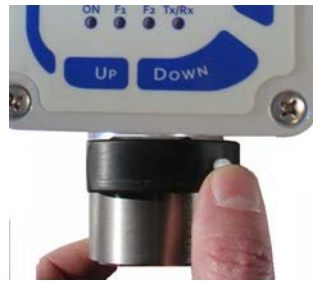
Fig. 2 From this position remove the magnet and the zero calibration procedure is terminated
