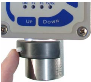
Fig. 1 Starting from this position, slowly move the magnet until reaching the final position in Fig. 2
