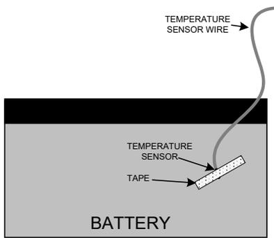
K21083M4 and K21084M4 models have a temperature compensation sensor held in place on the power supply chassis with adhesive tape. The tip of the sensor must be fitted to one of the batteries with the tape supplied for correct temperature compensation.
