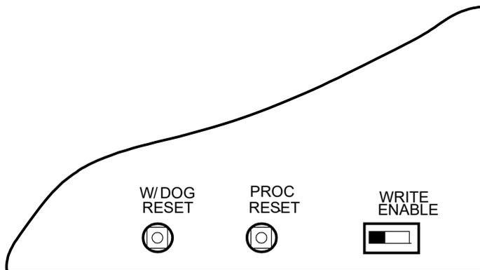
Internal controls on detection part of control panel
